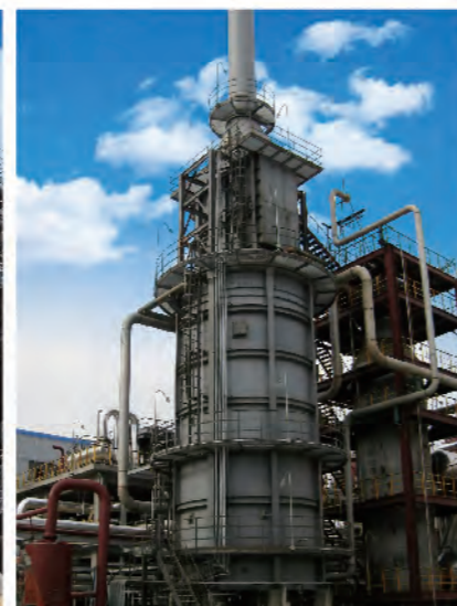
山东荣信25万吨/年甲醇装置预热炉 Pre-heating furnace for 250,000 t/y methanol plant of Shandong Rongxin Group
