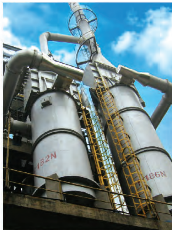
四川维尼纶天然气制乙炔项目天然气及氧气加热炉 Natural gas heater and oxygen heater for natural-gas-to-ethanol project of Sichuan Vinylon Plant
