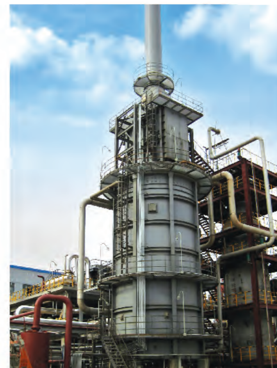
石家庄金石集团合成氨项目加热炉 Heater for synthetic ammonia project of Shijiazhuang Jinshi Group
