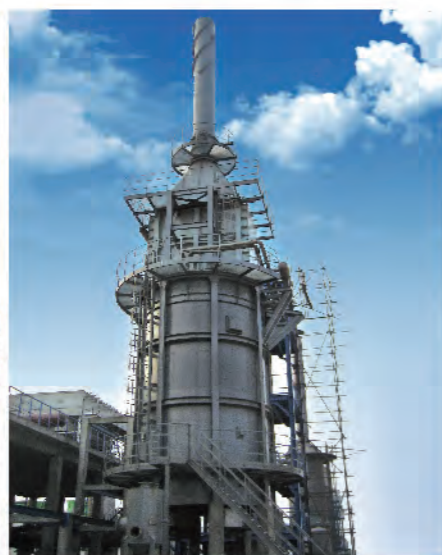
河北邢台旭阳焦油加工项目焦油管式炉 Tubular heater for tar processing project of Xingtai Coal Chemical Co., Ltd., Xu Yang, Hebei.
