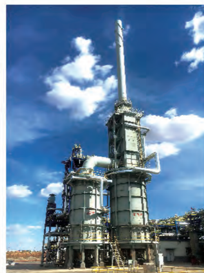
内蒙伊泰120万吨煤制油尾气制氢加热炉 Inner Mongolia yitai group 1200000tons/y coal-to-oil gas heating furnace for hydrogen production
